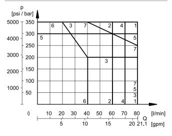
\* Performance obtained for a valve with A and B lines connected the one to the piston-side chamber and the other to the rod-side chamber of a double-acting cylinder with area ratio 2:1.
