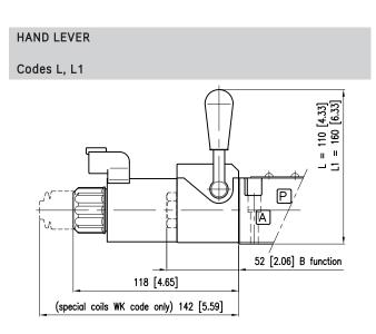
The lever device is always placed on side A, with the exception of the valves type HDS3-TB.
