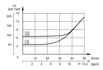
Pressure drops with flow  $A \rightarrow P$ . Obtained with  $Q_B = 0$ (de-energised coil - no current)
