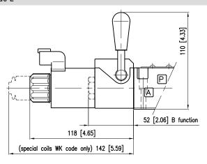
The lever device is always placed on side A. Valves with WK coils are equipped with the boot for solenoid tube protection.
