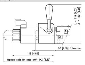
The lever device is always placed on side A, with the exception of the valves type  $\mbox{HDS3-TB}.$
