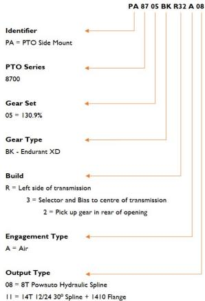
I I K = 14T 12/24 30° Spline + 1410 Flange + HD Output Bearing 23 = 8T Ø36 DIN 5462 Spline - Female and DIN Mount
