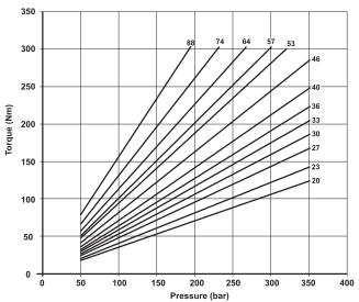
NOTE: this is typical torque date with an assumed mechanical efficiency of 90%
