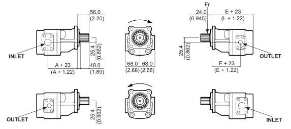
Maximum Radial Load (Fr) at 24.0 (0.945) from Mounting Face = 9000N (2025 lbf) The Outboard Bearing option is only available with the ISO 7653 Mounting Flange
