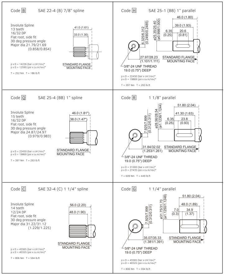
\* p = pressure, D = displacement. The stated values must not be exceeded.
