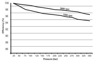
NOTE: These are actual volumetric efficiences measured on a 34 cc/rev pump.
